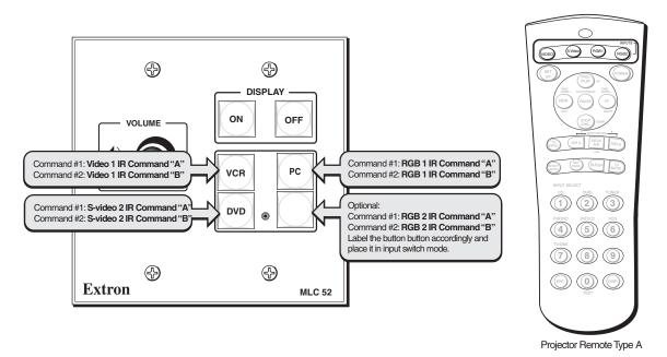
Programming an MLC 52 VC model with a projector remote control type A
